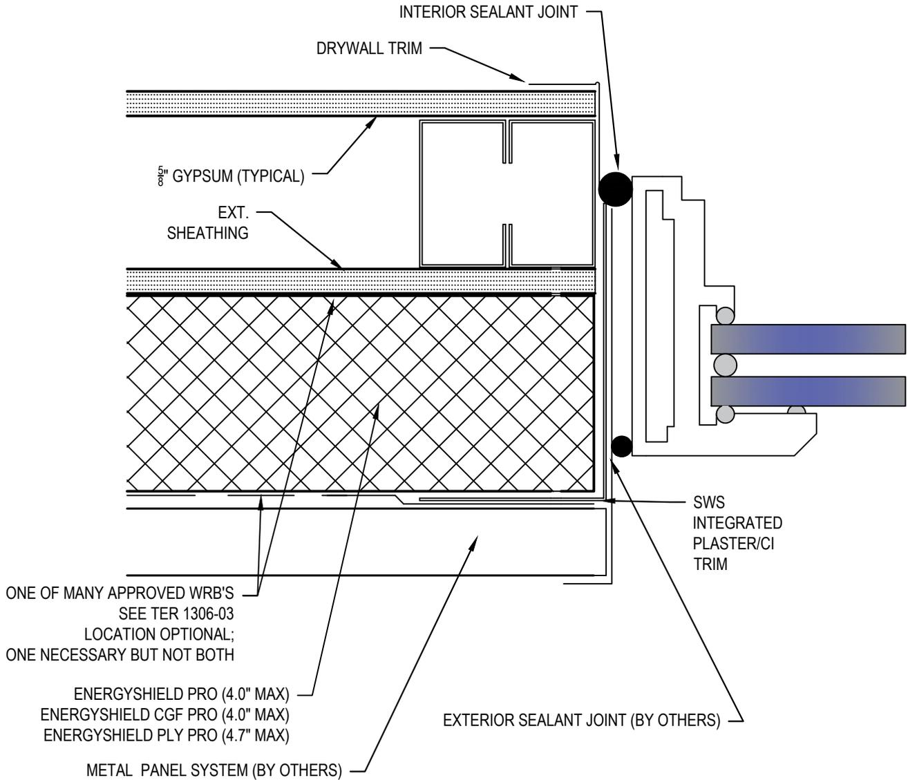
NOTE: WHEN ACM'S ARE USED, A MAXIMUM 2.25" AIR GAP BEHIND CLADDING IS APPROVED.
