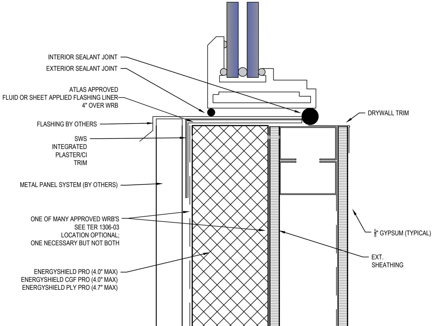
NOTE: WHEN ACM'S ARE USED, A MAXIMUM 2.25" AIR GAP BEHIND
