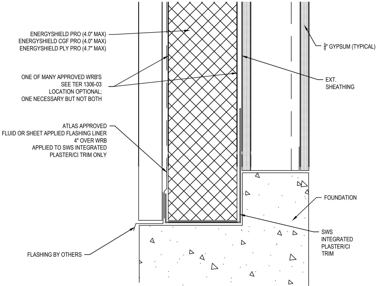
NOTE: WHEN ACM'S ARE USED, A MAXIMUM 2.25" AIR GAP BEHIND CLADDING IS APPROVED.
